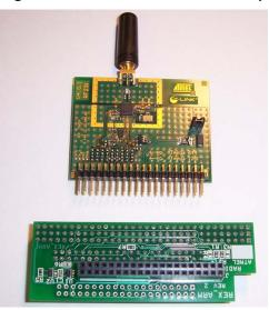
Figure E-1-3 AT91SAM7X-EK with REB/REX\_ARM Connected
